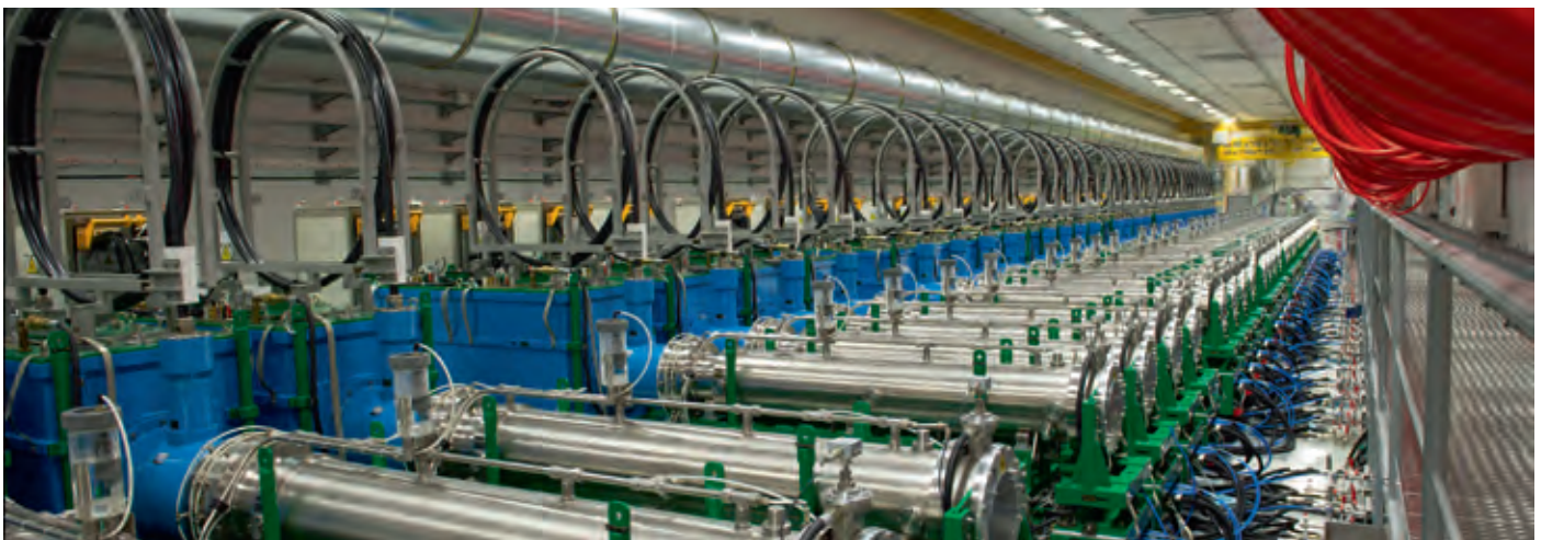
Airix flash x-ray radiographic machine installed in the EPURE facility © CEA/DAM
